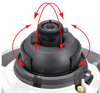
Sony Patented Ball-Joint Lens Mount
